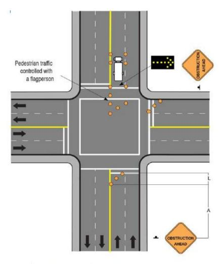
Placement of Temporary Traffic Control Devices
